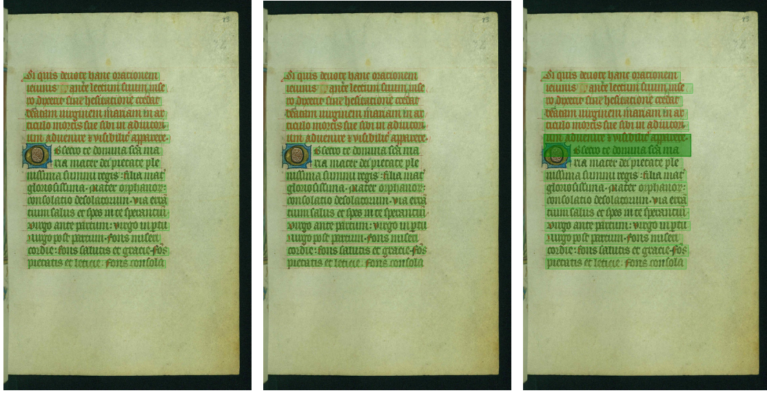
Fig. 4 Predictions of a page from Horae dataset: Doc-UFCN on the left, dhSegment in the middle and ARU-Net on the right. Doc-UFCN and dhSegment output similar results while ARU-Net shows thicker lines and two mergers of two lines (one is highlighted in dark green).
